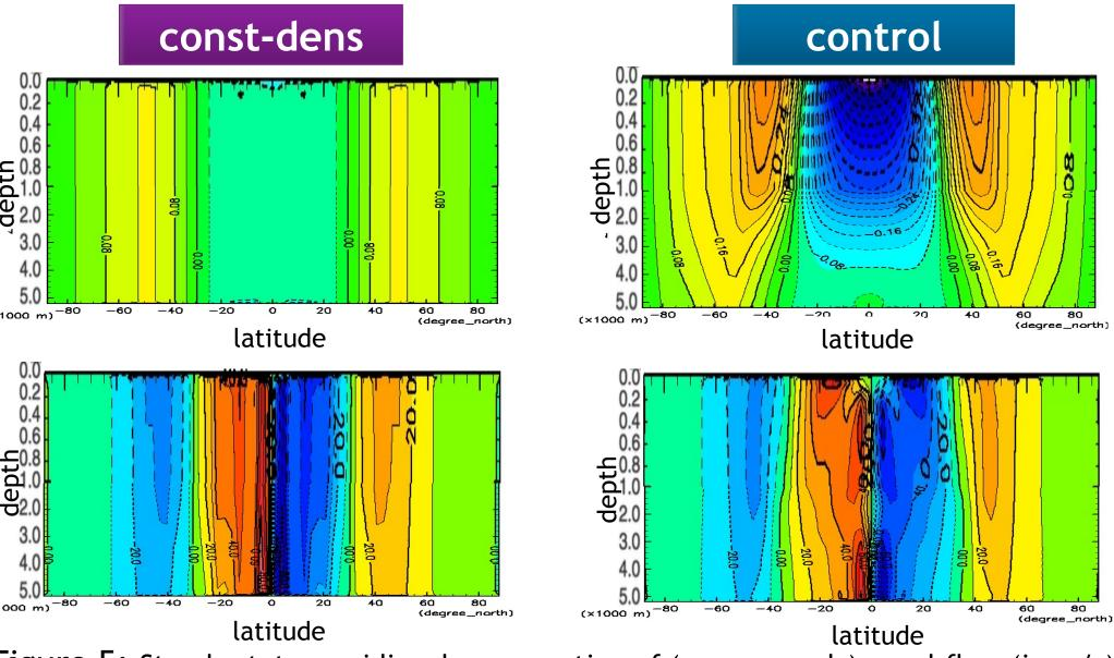
Figure 5: Steady state meridional cross section of (upper panels) zonal flow (in m/s), (lower panels) Eulerian-mean overturning circulation (in Sv)
